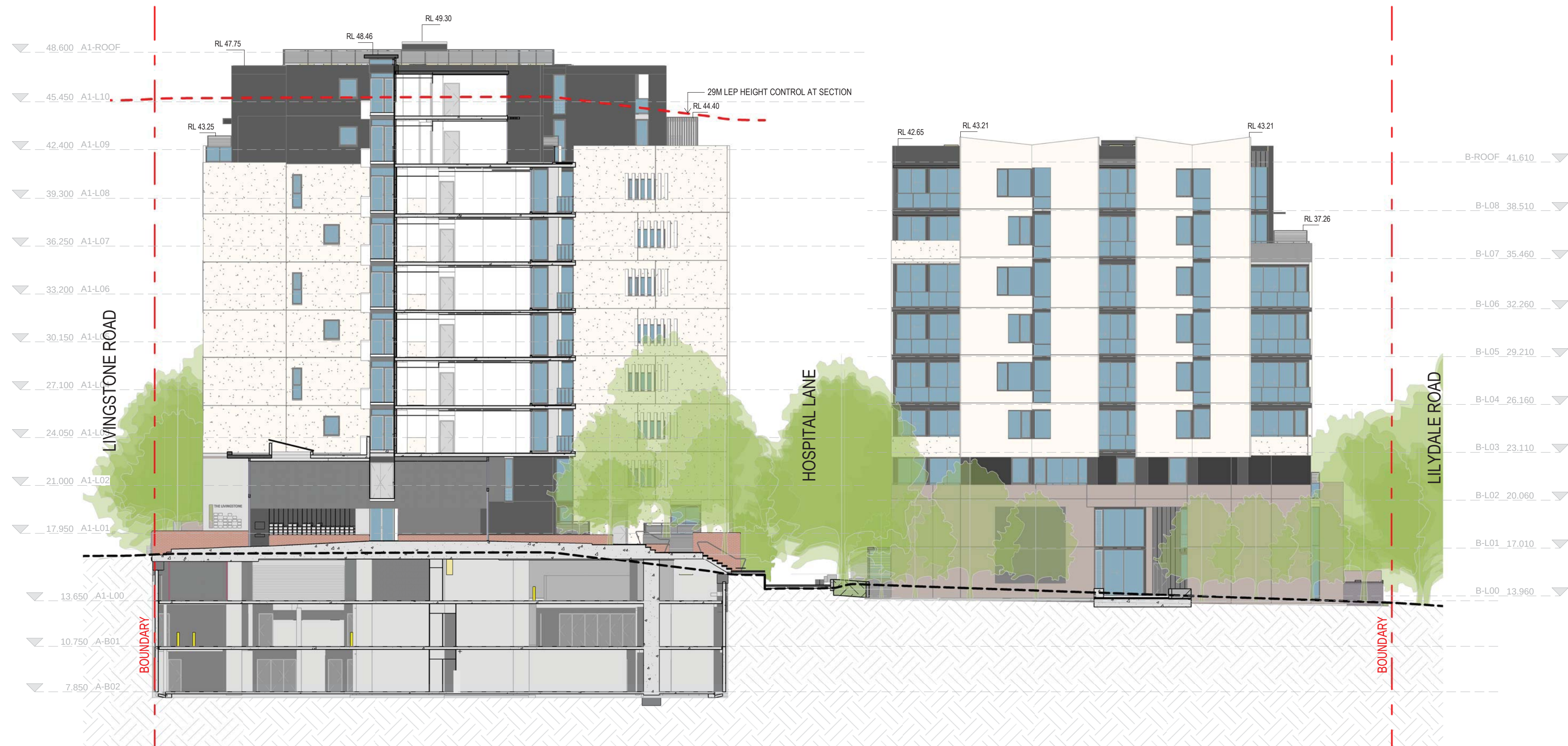
2 Section through Building A with Building B South Elevation 1 : 200
